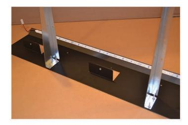
3. Position the Plexi Marquee in front of the metal mounting brackets; position and secure the top hole on each side of the marquee to the top hole on the metal mounting brackets using #8 black machine screws with black washers on the front side face of the plexi.
